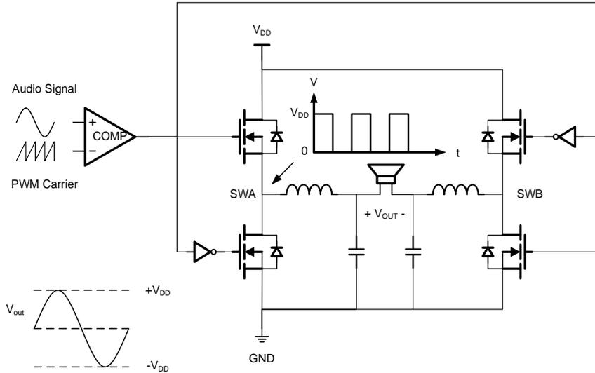
**Figure 3: MPQ7795-AEC1 BTL Class-D Amplifier**
