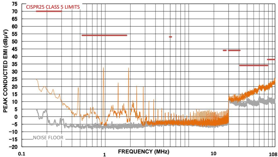
Figure 6: EMI Results for CISPR 25 Class 5 Peak Conducted Emissions
