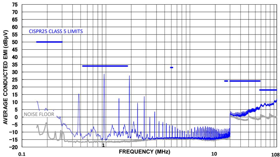
Figure 7: EMI Results for CISPR 25 Class 5 Average Conducted Emissions
