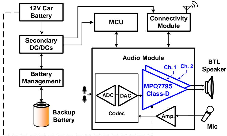
Figure 2: E-Call System (Simplified Block Diagram)
