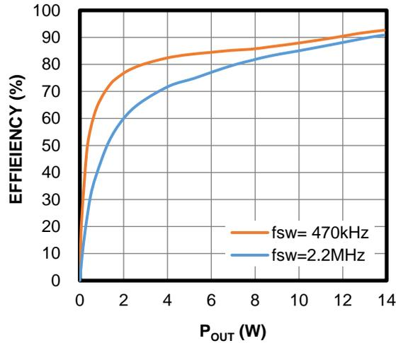
Figure 4: MPQ7795-AEC1 Efficiency Curve
