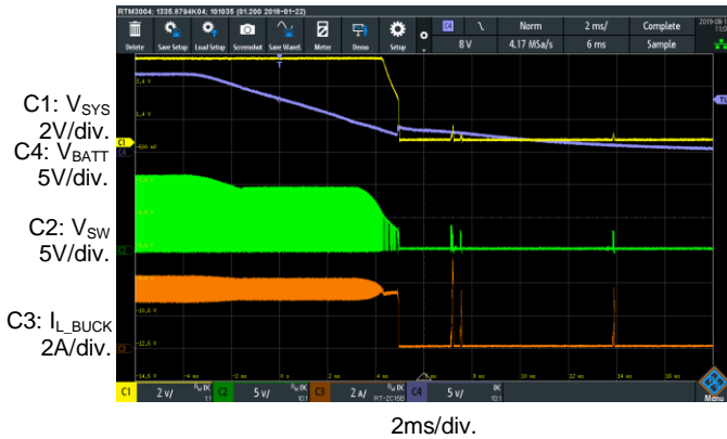
Figure 159: SCP Steady State
