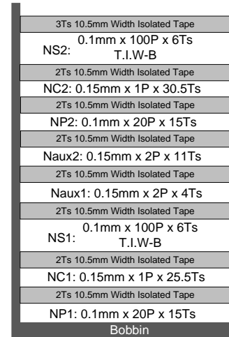
Figure 10: Winding Diagram
