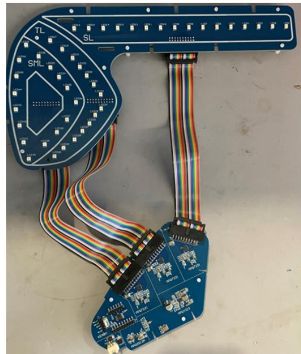
Figure 1: EVQ7221-TL-00A Tail Lamp Control Board and Tail Lamp Board
