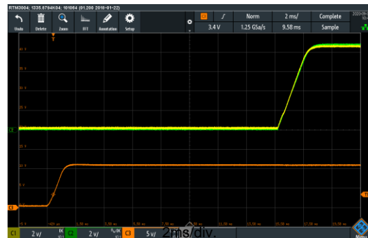
Figure 32: Start-Up through V_{IN} (MPQ2022)
