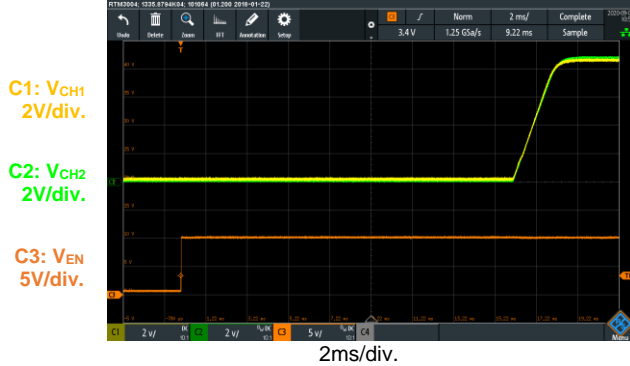
Figure 34: Start-Up through EN (MPQ2022) I_{LOAD} = 300\text{mA} (one channel)
