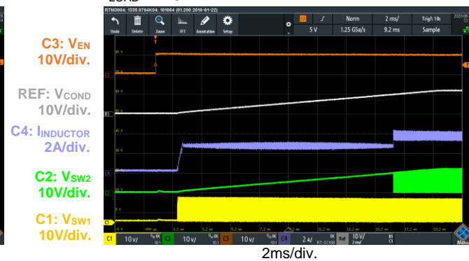
Figure 21: Start-Up through EN (MPQ8875A)
