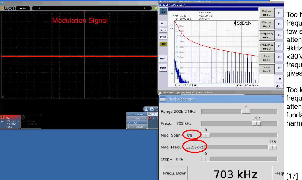
Too high a modulation frequency makes only a few spurs with little attenuation. For the 9kHz RBW area <30MHz, a modulation frequency of about 9kHz gives best results.
