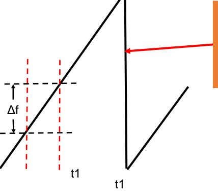
The df/dt here is high or infinity, which is good. However, the abrupt frequency change often creates additional output ripple in fixed frequency designs.
