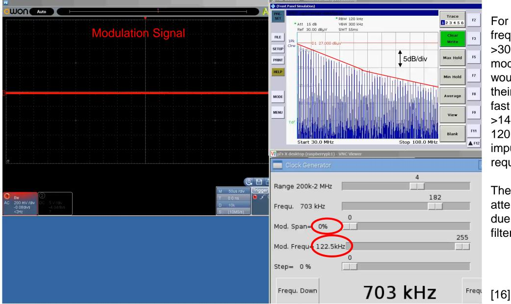
For the 120kHz RBW frequency range, >30MHz high modulation frequency would be best because their spurs still "move" fast enough against the >14.4GHz/s that the 120kHz RBW filter impulse response requires.
