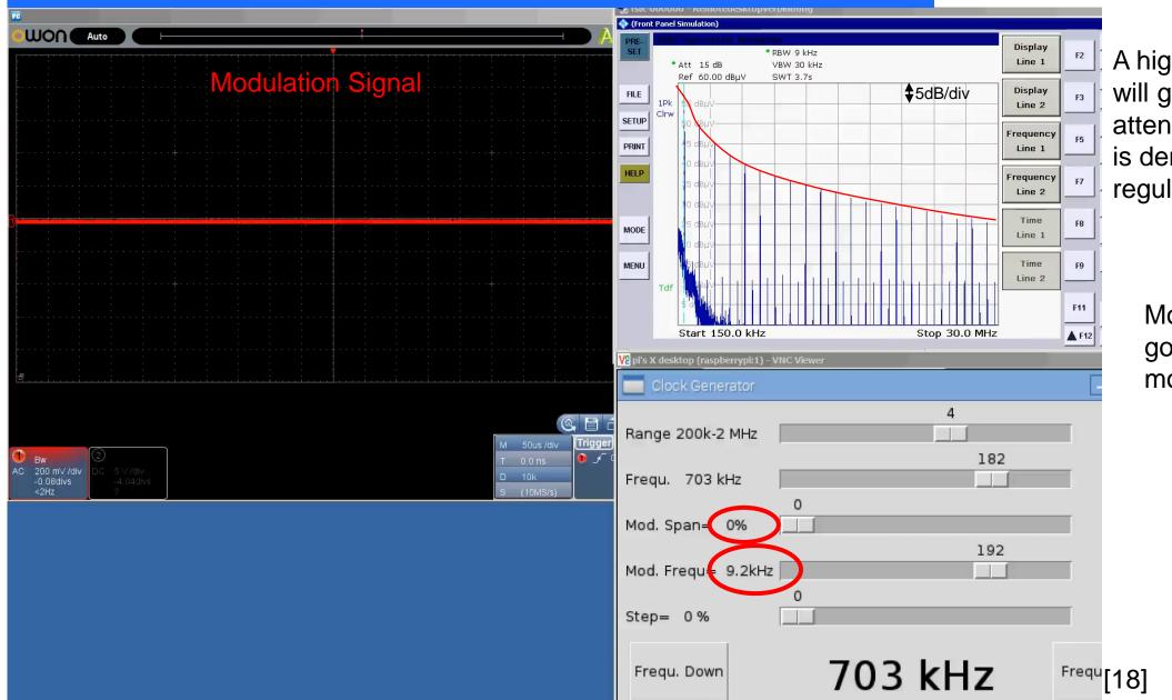
A high modulation span will give good attenuation results, but is demanding on the regulation loop.
