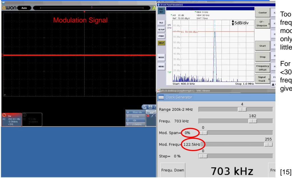
Too high modulation frequency = low modulation index makes only a few spurs with little attenuation.
