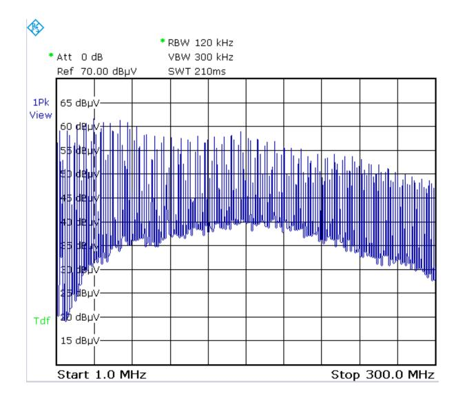
The typical PSU switch excitation source creates a flat periodic "fence" of spurs in the frequency domain, spaced by the switching frequency.
