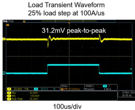
Figure 5. Load Transient Waveform of the Core Rail.
