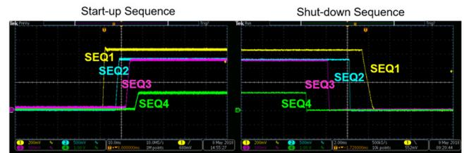
**Figure 4. Power-Up and Down Sequence**
