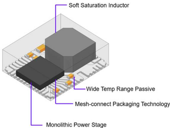
**Figure 2. Typical Structure of MPS Power Modules**
