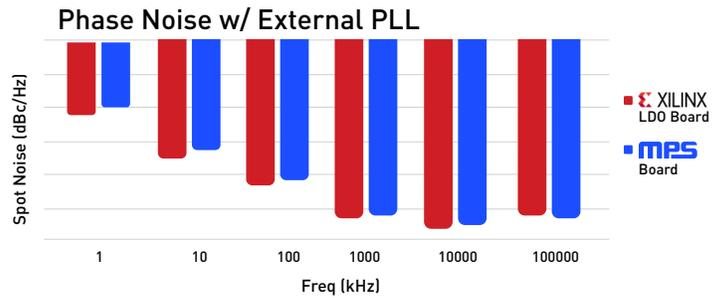
Figure 11. Comparison of Phase Noise of External PLL
