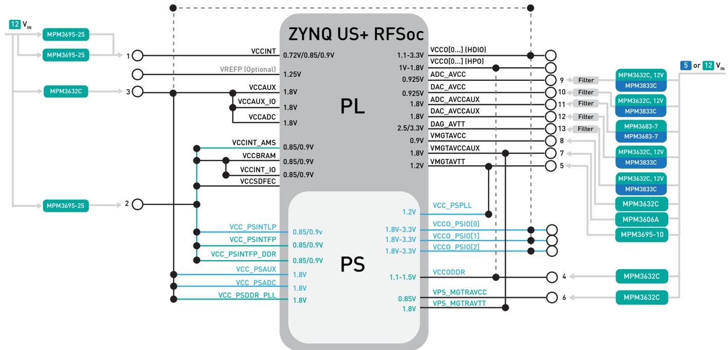
Figure 1. MPS Power Solution for Zynq UltraScale+ RFSoc
