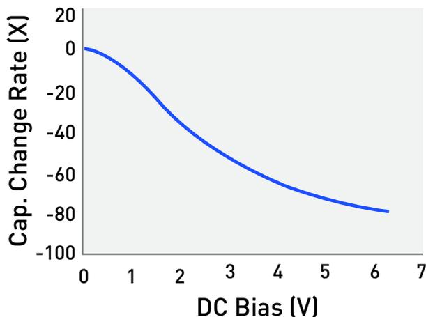
Figure 6. Typical Ceramic Capacitor Derating Curve at DC Bias Branch
