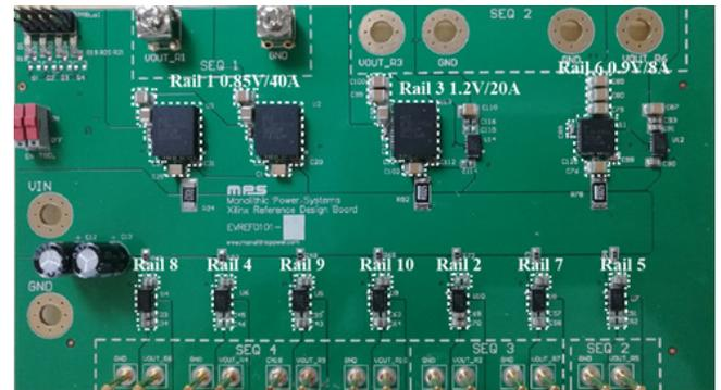
**Figure 3. Reference Design Board for Zynq UltraScale+ RFSoc**
