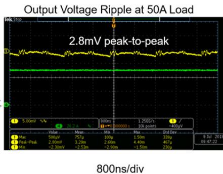
Figure 6. Output Voltage Ripple of the Core Rail.
