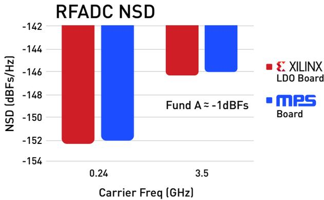
Figure 9. Comparison of RFADC NSD Results
