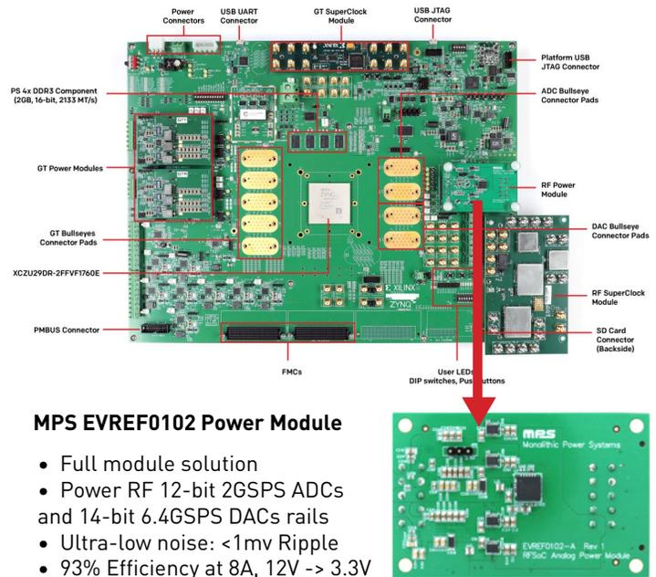
Figure 7. EVREF0102 Ultra-Low Noise Power Supply Module
