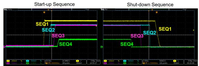
**Figure 4. Power-Up and Down Sequence**
