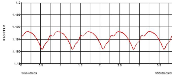
**Fig. 3 Output Voltage Ripple of the MPM3833C with One 22uF Output Capacitor**
