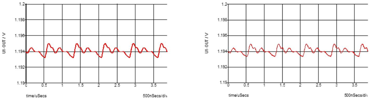
**Fig. 4 Output Voltage Ripple of the MPM3833C with (a) 4x22uF Output Capacitors and (b) 5x22uF Output Capacitors**
