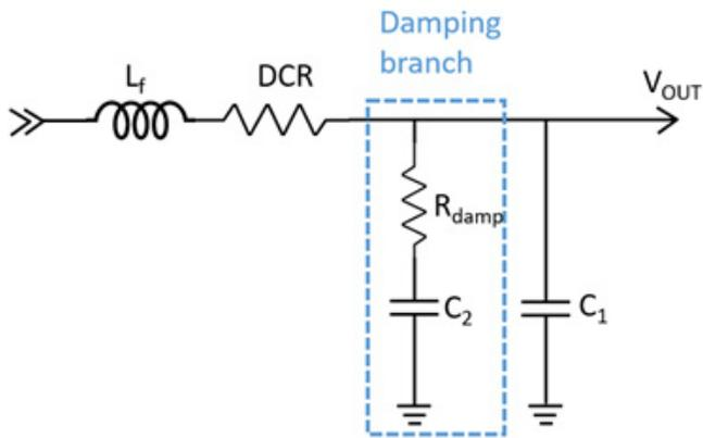
**Figure 5. Second Stage LC Filter with Parallel Damping Branch**
