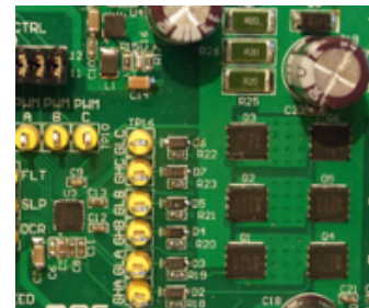
Pre-Driver plus 6 MOSFETs: 50mmx30mm
