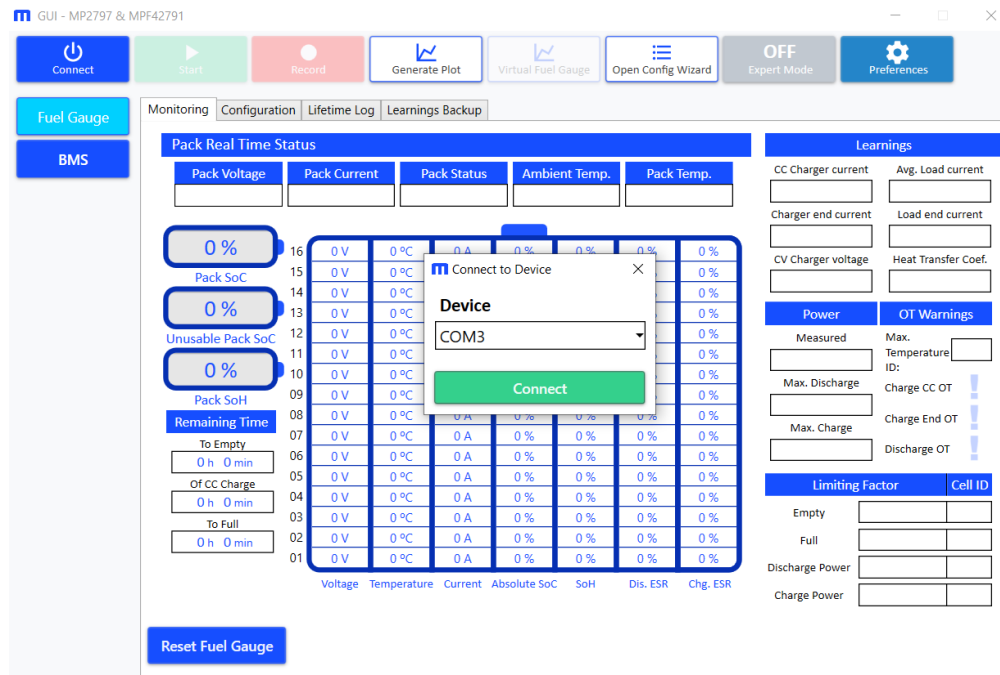
Figure 29: EVB Connection to the PC
