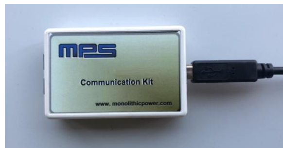
Figure 19: USB to UART Communication Interface (FT485R-KIT)
