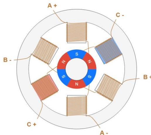
Figure 1: Stepper Motor
