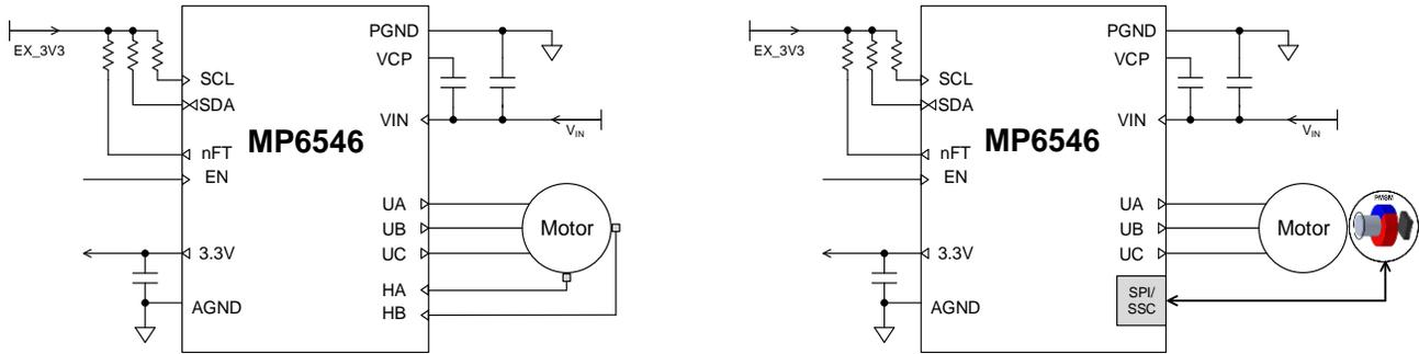
**Figure 6: Input Mode (Left: Hall Sensor, Right: Magnetic Angle Sensor)**
