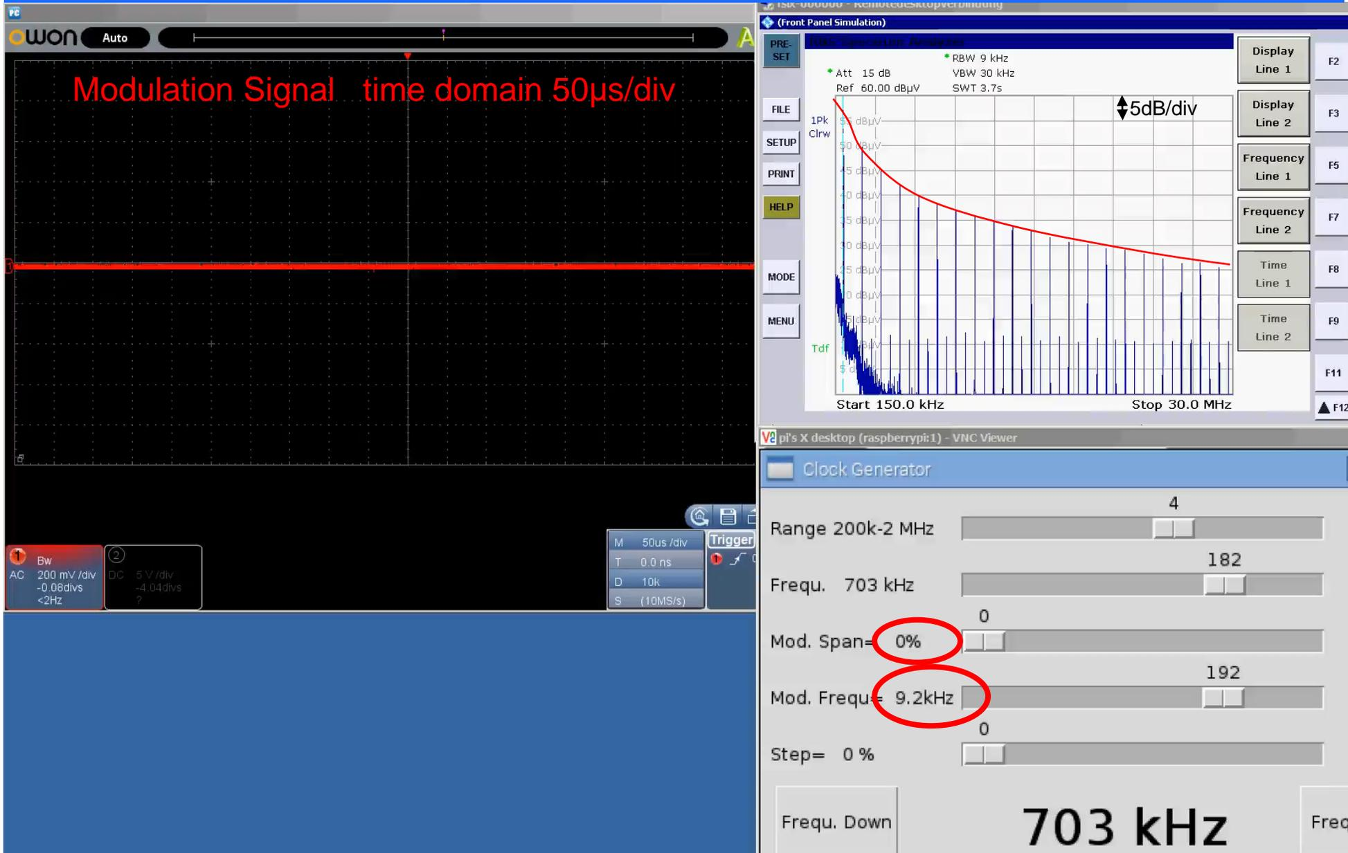
A high modulation span will give good attenuation results, but is demanding on the regulation loop.
