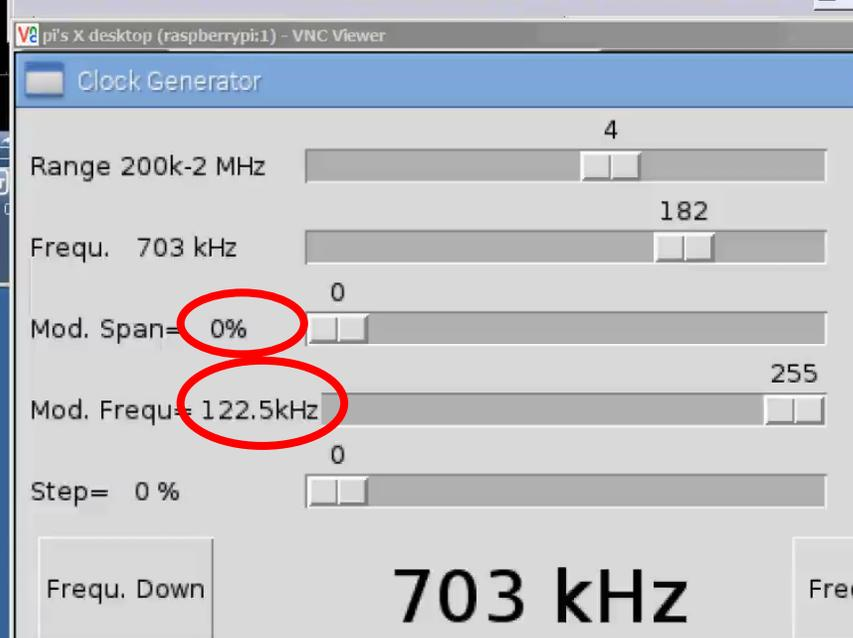
Too high a modulation frequency makes only a few spurs with little attenuation. For the 9kHz RBW area <30MHz, a modulation frequency of about 9kHz gives best results.
