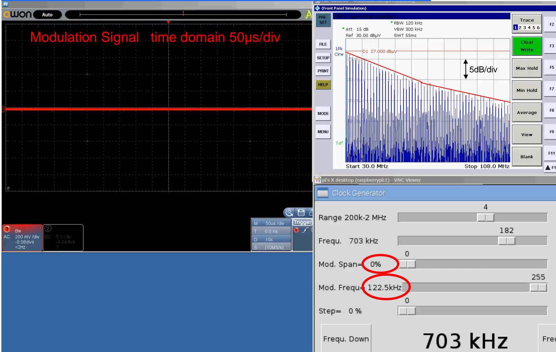
For the 120kHz RBW frequency range, >30MHz high modulation frequency would be best because their spurs still “move” fast enough against the >14.4GHz/s that the 120kHz RBW filter impulse response requires.
