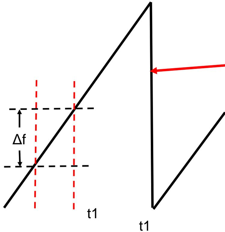
The  $df/dt$  here is high or infinity, which is good. However, the abrupt frequency change often creates additional output ripple in fixed frequency control loop designs.
