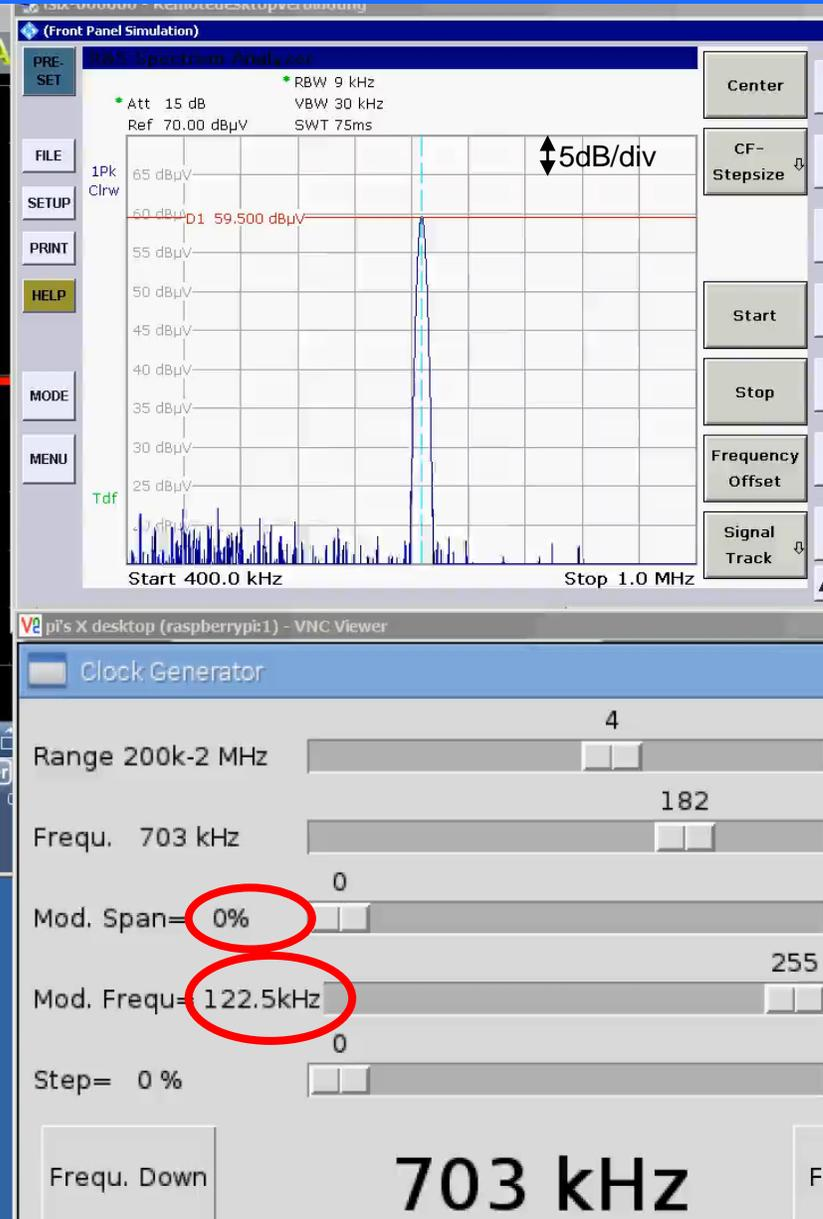
Too high modulation frequency = low modulation index makes only a few spurs with little attenuation.
