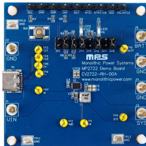
Figure 7: Prototype of 15W, DRP USB Type-C Solution with the MP2722
