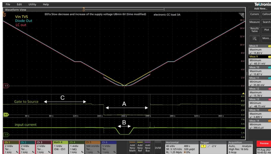
Figure 6: LV124 E07a Test ( I_{LOAD} = 3A , 180cm Harness)
