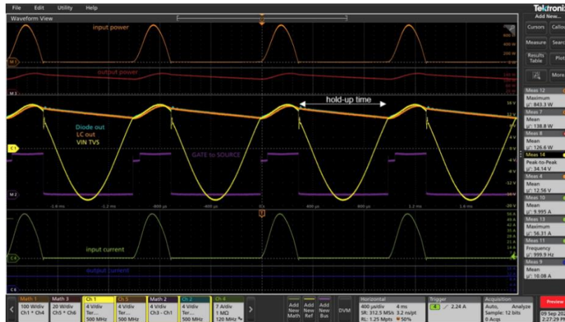
Figure 7: LV124 E06 Test ( V_{SOURCE} = 34V_{PEAK\_PEAK} , Superimposed AC Rectification, FREQ = 1kHz, I_{LOAD} = 10A , P_{IN} = 843W_{PEAK} , 180cm Harness)
