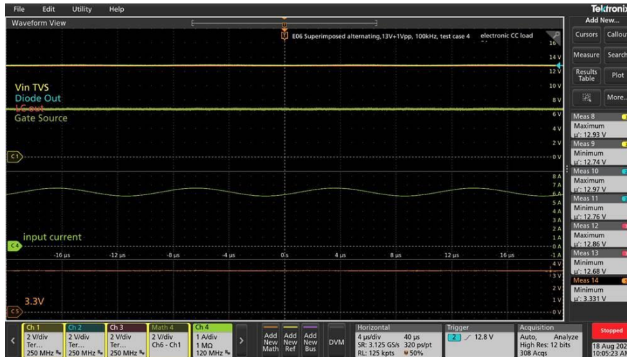
Figure 8: LV124 E06 Test (AC Rectification, FREQ = 100kHz, I_{LOAD} = 6A, 2cmx180cm Harness)
