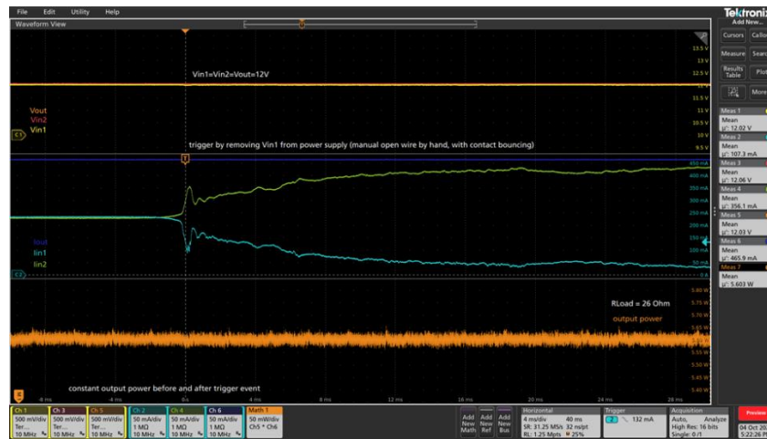
Figure 22: System Behavior (4ms/div. Time Base, P_{LOAD} = 5.6W ) (4)
