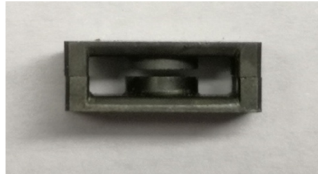
Figure 7: ER Core with an Air Gap
