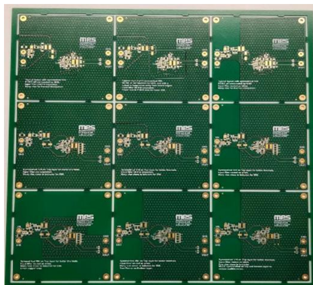
Figure 1: PCB Panel with Nine Different Layouts
