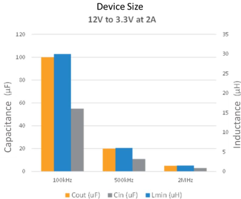
Figure 1: Required Peripheral Device Parameters
