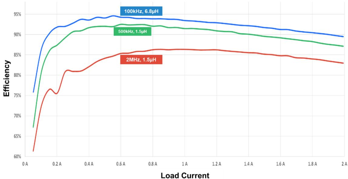
Figure 2: Efficiency Curves at Different Frequencies
