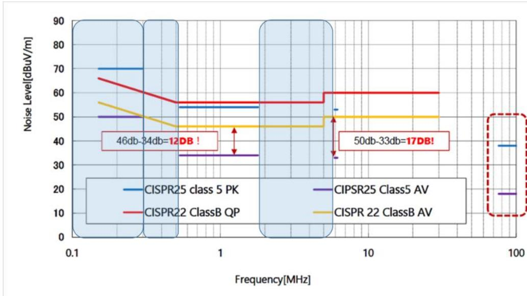
Figure 3: CISPR25 Class 3 CE Limit Standard Chart
