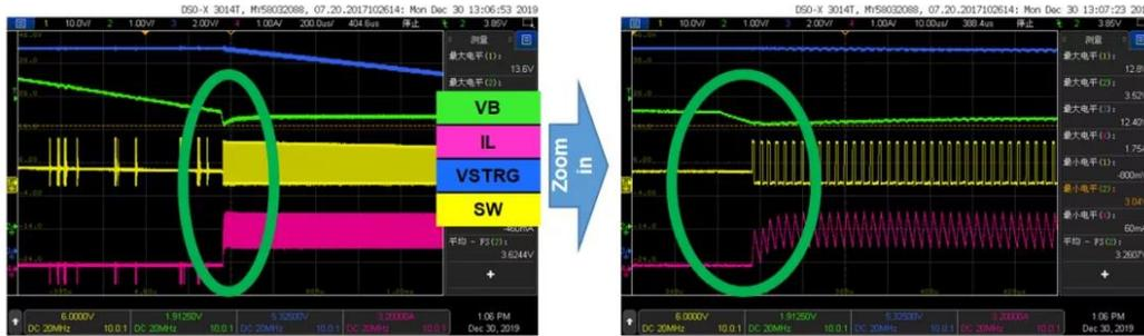
Figure 8: MP5515 Shutdown Transition Waveforms
