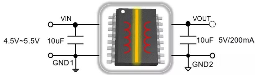
Figure 4: MID1W0505A Typical Circuit
