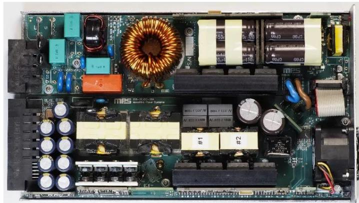
Figure 1: MPS Solution for 3kW Power-Level Isolated Power Supply
