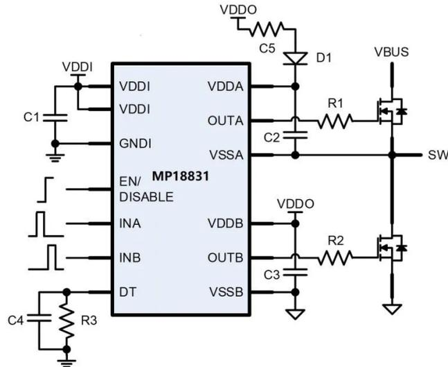
Figure 2: MP18831 Typical Application Circuit
