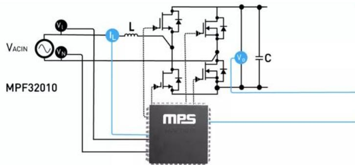
Figure 3: MPF32010 Integrates Entire Control Loop
