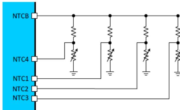
Figure 2: Four-Channel NTC Sampling
