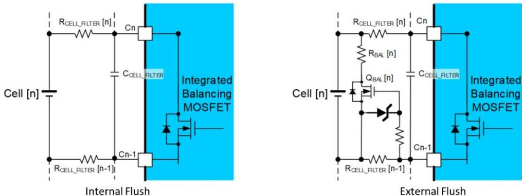
Figure 3: Cell Balancing Reference Circuit
