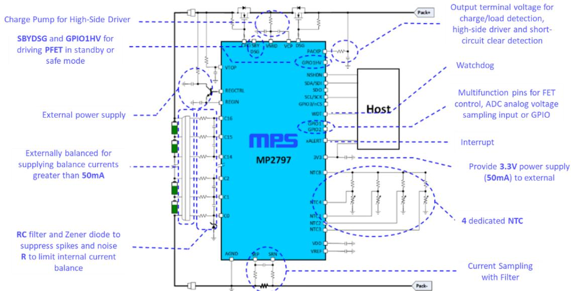
Figure 4: MP2797 Typical Application Circuit
