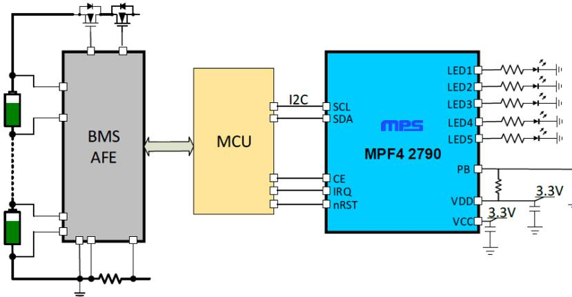
**Figure 6: MPF42790 Typical Application Circuit**
