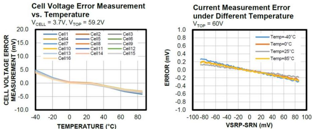
Figure 1: Cell Voltage Measurement and Current Measurement Error Curves
