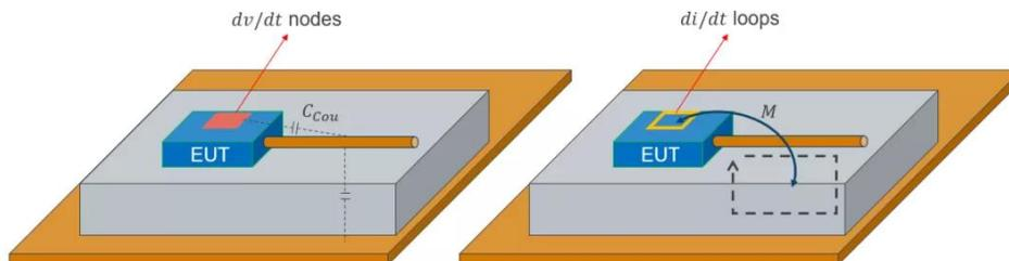
Figure 8: EMI Noise Generated by Electric Field Coupling and Magnetic Field Coupling
