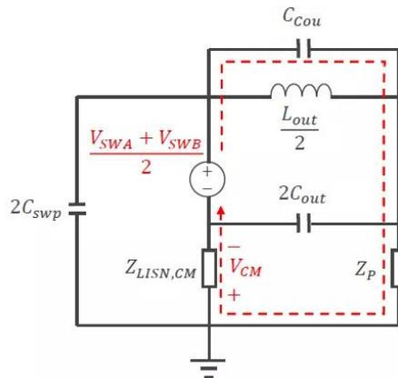
Figure 9: Modified EMI Model for Electric Field Coupling
