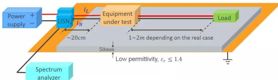
**Figure 2: Long-Term Load Test Device Based on CISPR 25**
