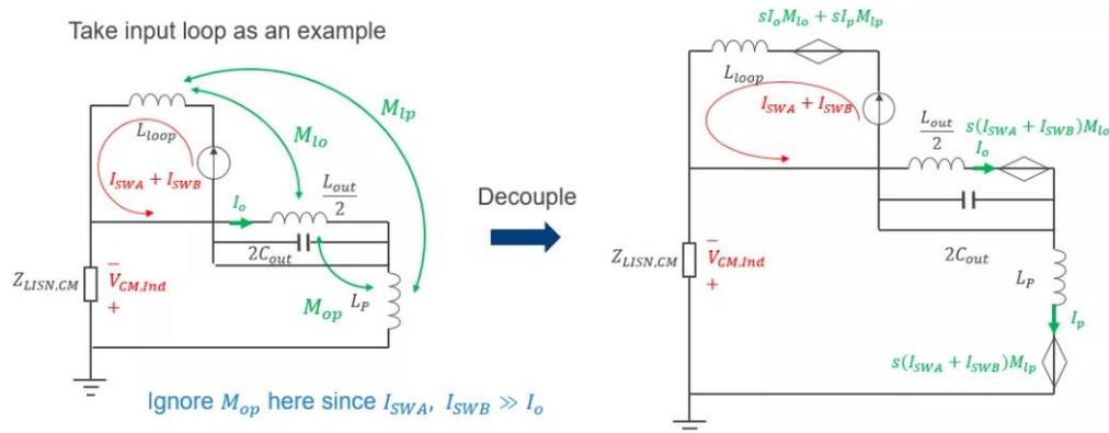
Figure 10: Modified EMI Model for Magnetic Field Coupling
