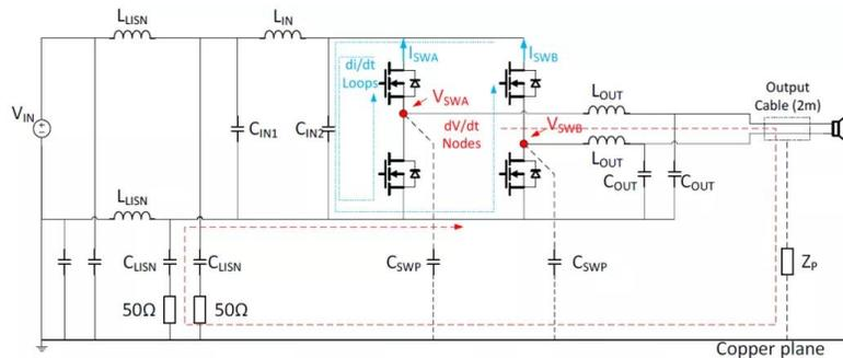
**Figure 4: CM Noise Path of Class-D Power Amplifier**
