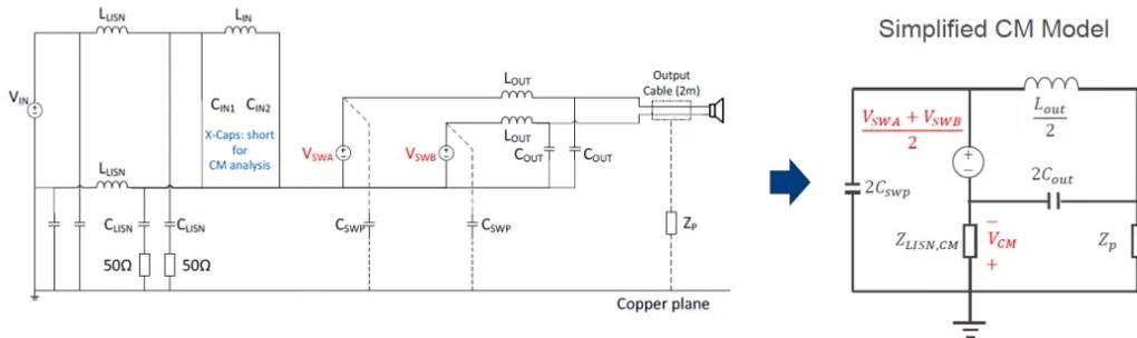
Figure 7: Analysis of the Common-Mode Noise Voltage Source
