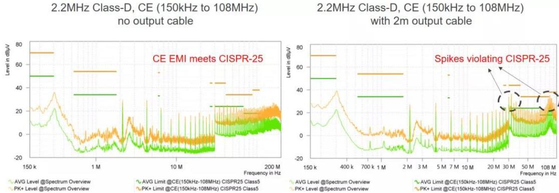
**Figure 3: Long-Term Load Comparison (No Output Cable and 2m Output Cable)**
