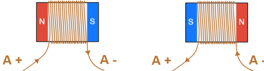
Figure 8: Direction of the Magnetic Field based on the Direction of the Coil Current
