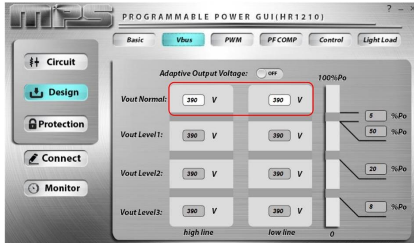
Figure 2: HR1210 Adjustable PFC Output Voltage
