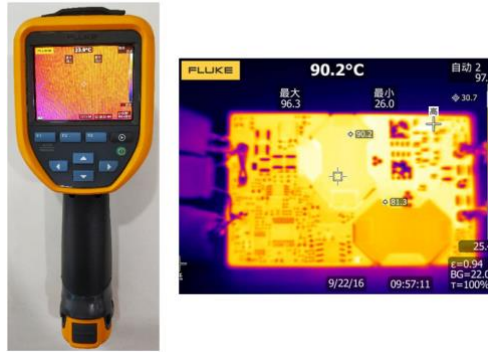
Figure 9: Measuring Inductor Temperature Using a Thermal Camera
