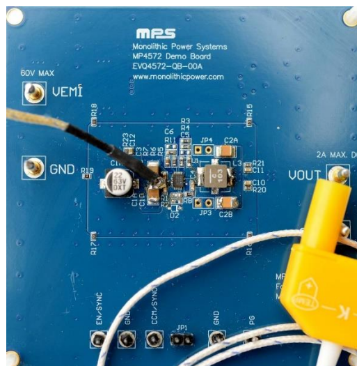
Figure 3: Soldering a Thermocouple to the PCB
