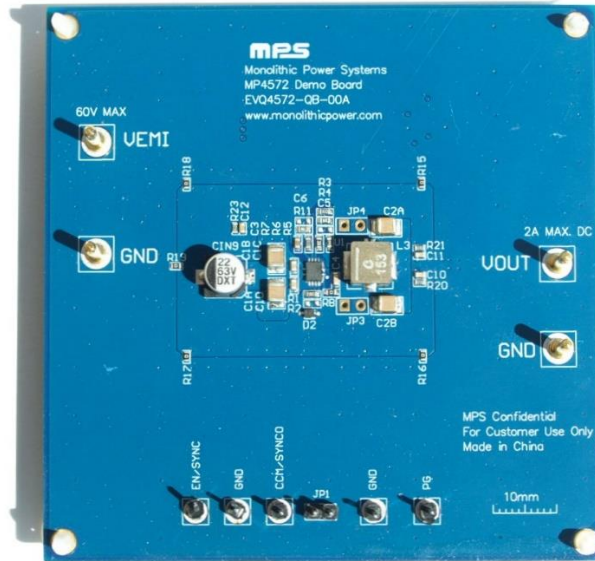
Figure 2: EVQ4572-QB-00A 4-Layer Evaluation Board (8.9cmx8.9cm)
