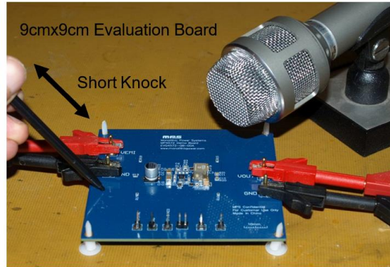
Figure 5: Set-Up to Measure Audible Noise
