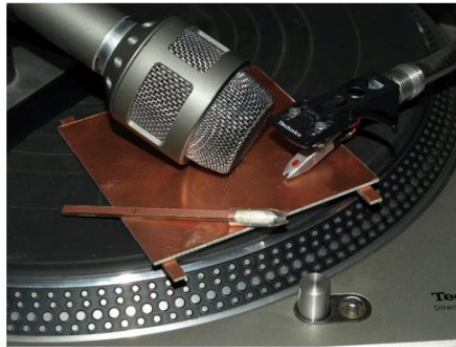
Figure 7: Turntable Set-Up to Measure Horizontal Vibration
