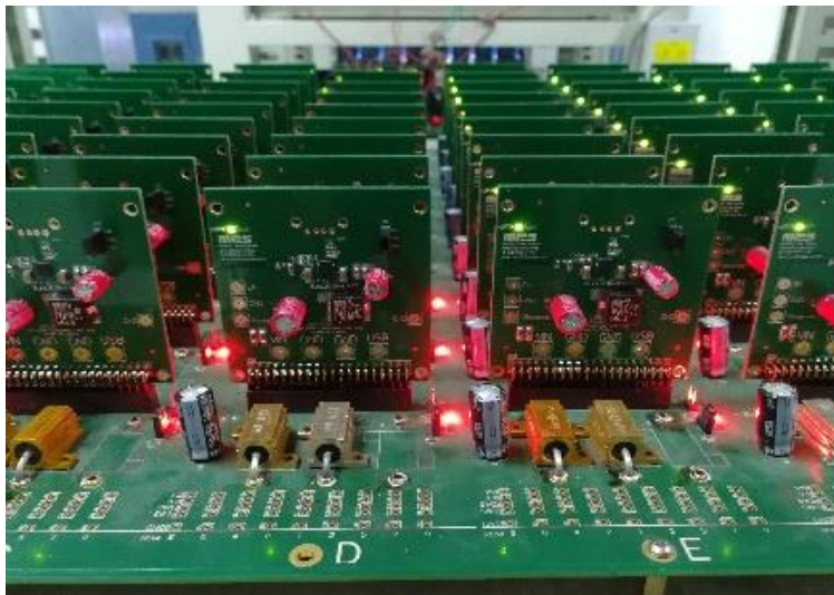
Figure 3: MPS Devices Under HTOL Test Operate Under Load Conditions
