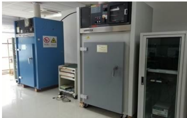
Figure 2: MPS HTOL Chambers
