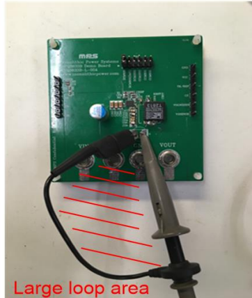
Figure 4: Ripple Measurement with Passive Probe
