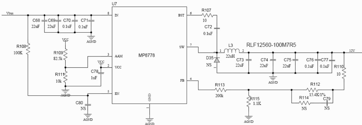
Figure 29—MP8778 DC/DC Converter
