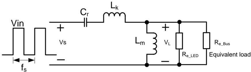
Figure 10B—Equivalent Circuit of MP4653 LLC Power Stage
