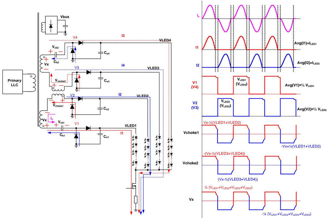
Figure 40—Choke+ Cap Balance Circuit and Operating Waveforms
