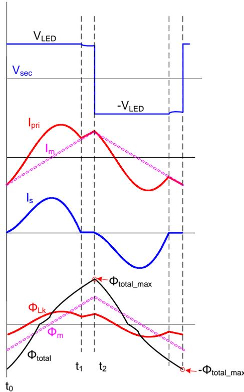
**Figure 37B—Waveforms of the LLC Power Stage at  $f_s < f_0$**
