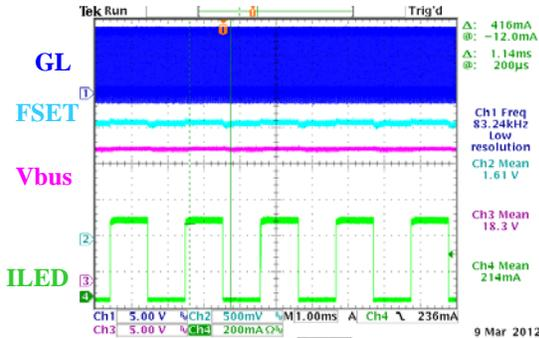
PWM+ Analog Dimming (A\_Dim=0.99V)
