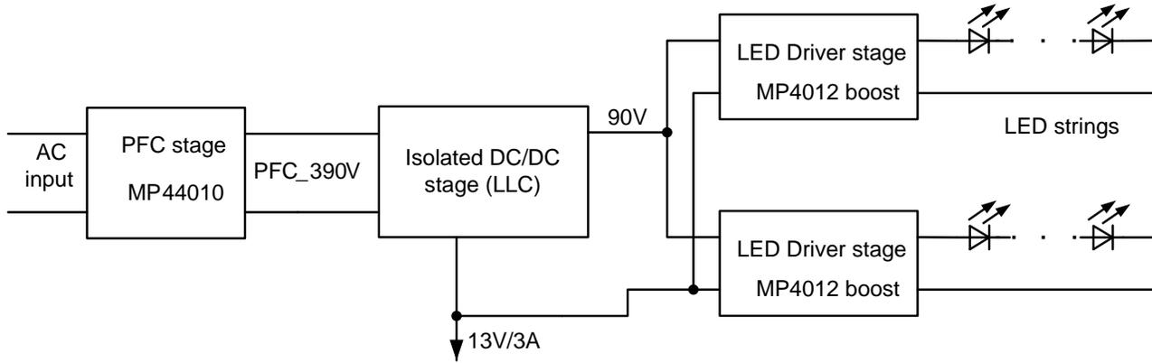
**Figure 2—Traditional 3-stage TV LED Driver Power Structure**
