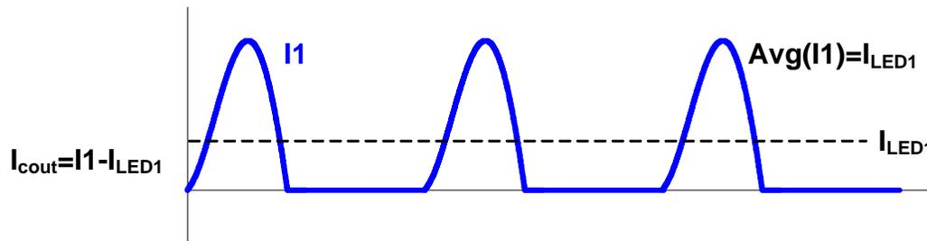
**Figure 41—Current though the Output Capacitors of LED Stage**
