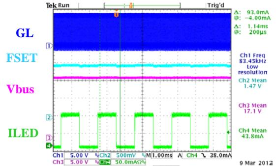
PWM+ Analog Dimming (A\_Dim=0.19V)
