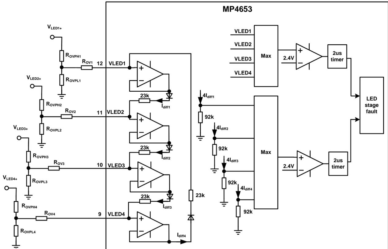
Figure 22—MP4653 LED# (#=1,2,3,4) Pins Protection Scheme
