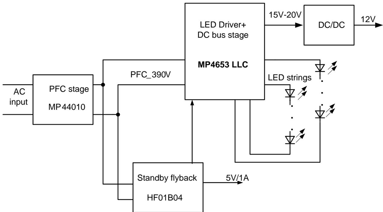
**Figure 1— MP4653-Based 2-stage TV LED Driver Power Structure**
