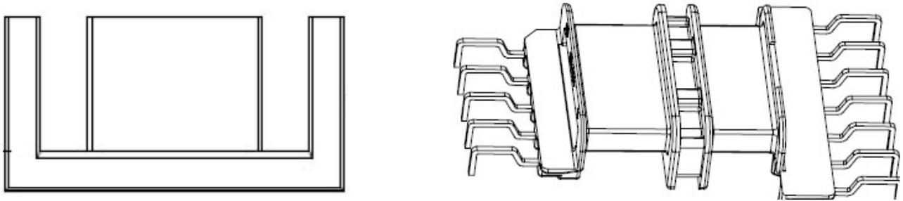
Figure 36—EFD Core and Its Bobbin with 2 Slots
