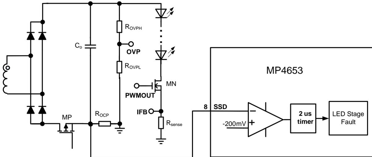
Figure 21—MP4653 SSD Function for Short Circuit Protection of the LED Stage
