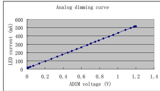
Analog Dimming Curve
