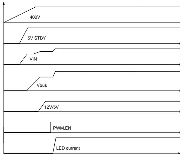
**Figure 13—MP4653 Power System and Start Up Sequence**
