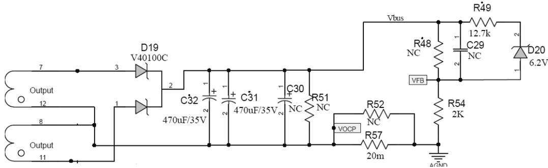
Figure 44—DC Bus Voltage Feedback
