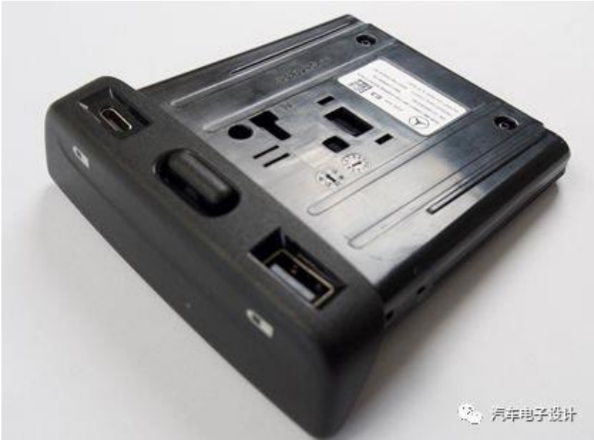
The entire module is wedge-shaped and thin for ease of insertion. This answers the question of putting ports in tricky places in the car. Quite a bit of thought went into this design.
