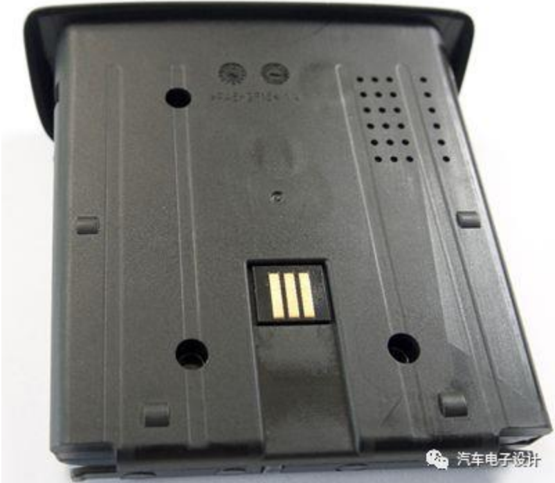
The input interface on the back of the module has three input ports.
